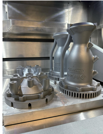
Figure 4 - Printed Engine and Swirl injectors inside the EP-M400S
