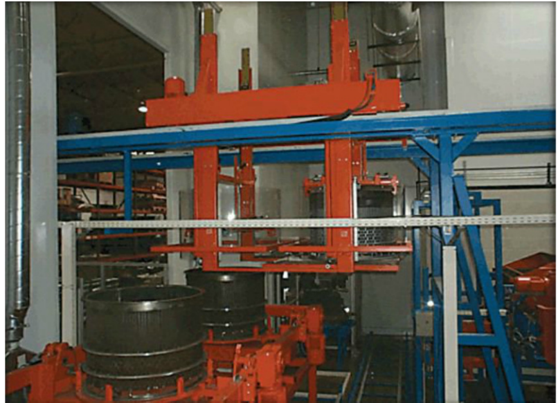
Dip spin hoist used to apply multi-layer, zinc-flake coating systems at SWD Inc. (above). Samples of fasteners and other components processed with these coatings at SWD (below).
