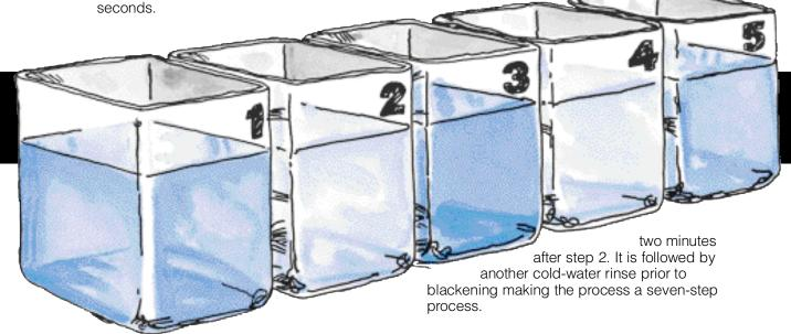
Blacken—Immerse for two to four minutes at room temperature in a 10% to 15% by volume solution of *InstaBlak* 333.
