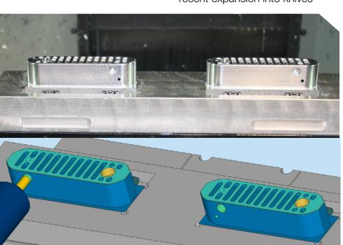
DoubleStar butt plates being machined
