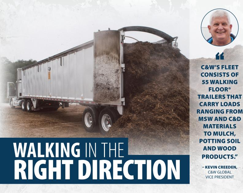
railers equipped with WALKING FLOOR® technology b. from Keith Manufacturing Co. have helped a Florida
