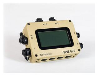
**Above:** The Protonex® SPM-622 Squad Power Manager is a tough and compact device which weighs less than a pound and enables military units to optimize power for multiple electronic devices.
