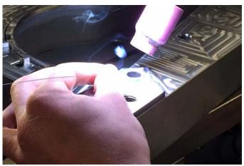
PLT offers Laser Deposit Welding services for the repair of mold components. Whether your repair request is for design changes, reconditioning of existing tooling, or manufacturing corrections, PLT can address your needs quickly and precisely. PLT's mold experience and welding techniques minimize the amount of post work necessary to return your mold into production.
