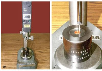
Fig. 6. Indentation measurement system: (a) rimfire copper-crusher test instrument; (b) indent being measured with depth indicator (courtesy of Olin Corporation)
