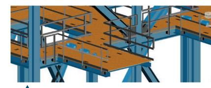
Grating features and fabrication extras (toe plate, anchor blocks, hatches, hinges, etc.) are included in the model.
