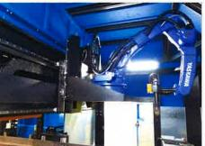
The latest 6 axes MOTOMAN robot, plus the 2 axes MOVING ROBOT BASE
