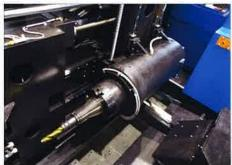
3 spindles with direct drive built-in motor enables a quiet, accurate, powerful and stable drilling / milling condition.
