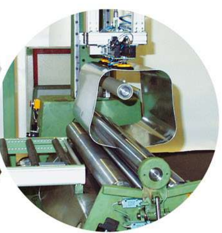
Automatic outfeeding of finished tank body
