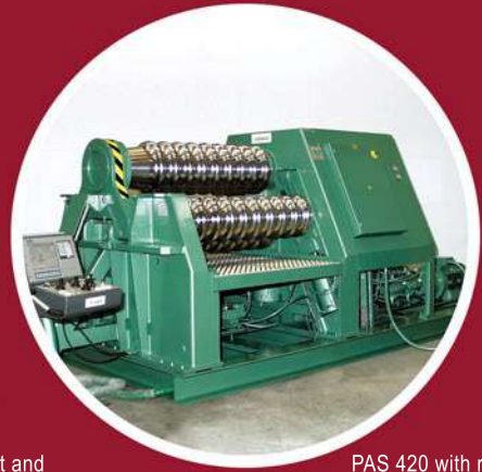
PAS 420 with rolls for bending of corrugated plates
