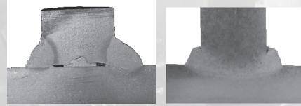
Stud Welding is an electric arc process where an arc is drawn between the base of the stud and the base metal creating the equivalent of a penetration weld in less than 1.5 seconds.
