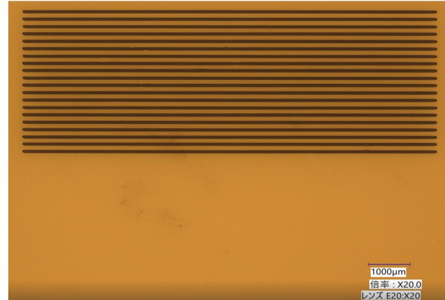
Comparison of Drawing Results at L/S = 50/50 \mu\text{m}
