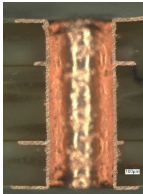
Cross section of 4-layer through-hole board Cross section of 8-layer through-hole board
