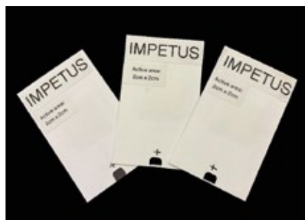
Fig. 3: Printed Zn-MnO 2 battery on paper, developed in the EU Horizon 2020 funded project IMPETUS
