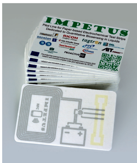
[Fig. 1]: Self-powered blood test cards developed within IMPETUS project using SaralBattery Inks in an integrated printing process (Source: IMPETUS project)
