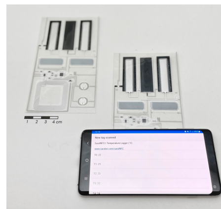
[Fig. 3]: Development of fully printed temperature logger using Saral Inks
