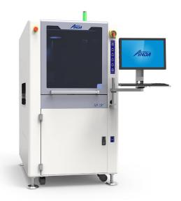
Plasma treatment removes static electricity and contaminants such as fine dust, oil, grease, microbial organisms, and both organic/inorganic compounds while also providing surface modification which facilitates adhesion of various coatings and/or adhesive materials. Additionally, plasma treatment promotes the flow of coatings for thin-film coating without other mechanical or chemical treatments required.
