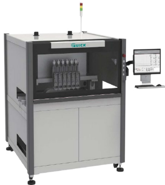
Hotbar Robot Automaterial loading and unloading pressure and temperature of six soldering heads closed-loop controls individually
