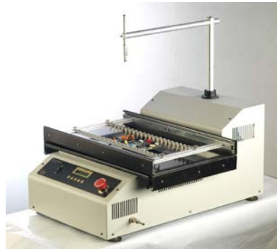
Manual Selective Soldering
