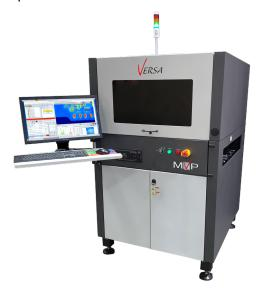
Uniquely, MVP's Versa system allows fast programming and the flexibility to fit into all the processes in the line: Paste Inspection, Pre-Reflow, Post-Reflow, Post-Wave and Selective Solder.
