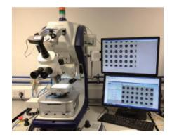
Figure 4: Test setup for BST testing. The wafer samples were secured using a vacuum wafer chuck.
