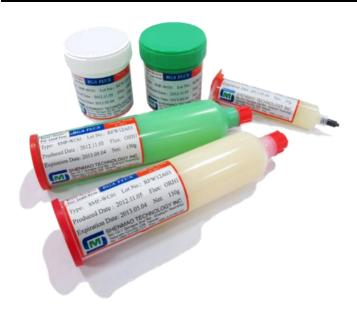
SHENMAO SMF-WB02 / SMF-WB51 Water Soluble Flux are made locally in the USA and with the same quality in 7 other world wide locations. It is said their Low Viscosity (easy to apply), High Tackiness (slump resistant), consistent printability for BGA and Micro BGA Ball Assemblies and excellent wash ability after high temperature reflow (255°C and 60 sec over 220°C) create highly reliable Solder Joints with ultra maximized Quality.
